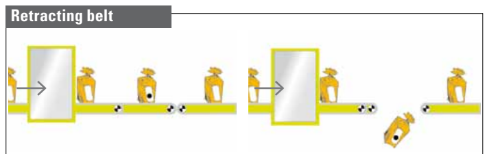
Separating systems To avoid the necessity of manual operator action in case of metal detection, the detectors can be combined with automatic separating systems. Since the design of such separating systems must consider a great variety of parameters (product distance, shape, size, nature, conveying speed, minimum ejection, function monitoring, etc.) S+S offers separating systems in various design versions.
